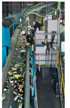
Segregation process of used beverage containers at a recycling facility
